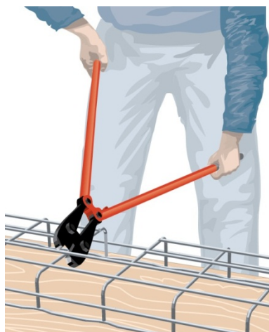
Figure 3-66 Cutting with Bolt Cutters
