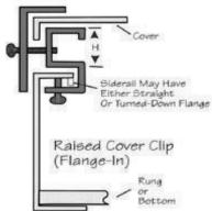
Cover stand-off clips provide a means to mount the cover above the tray side rail, allowing side ventilation. Cover stand-off clips should only be used with flanged covers and are available in various heights, offering a choice in the amount of open area for side ventilation. (Part # is for 1ea.)
